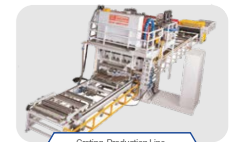
Grating Production Line
